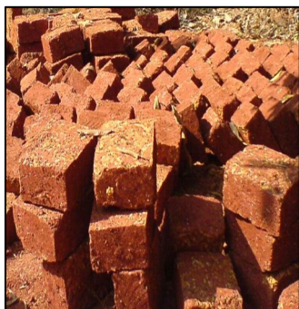
Laterite blocks mined in Goa (Source: Directorate of Mines and Geology, Goa, www.dmggoa.goa.gov.in/laterite.php )
