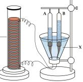
Figure 3: Experimental set-up for electrolysis.
