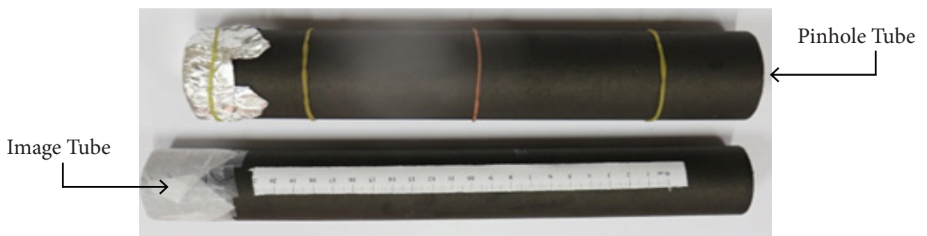
Figure 4 Image Tube (IT) and Pinhole Tube (PT)
