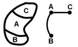
Note that the links need not be straight lines, it can be curved as well like the one in the network diagram drawn above.
